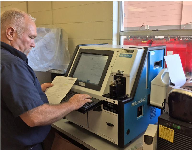
All the user has to do is insert a sample, input some basic information about the oil and equipment and the instrument performs up to four different types of analyses. These analyses provide a complete picture of the oil and powertrain condition.
